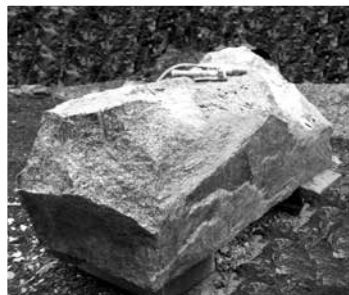
It starts by guessing what is excess and busting it off with shims and wedges . . .
