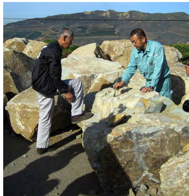
LEFT TO RIGHT, JUNJI AWATA AND TETSURO TANABE MARKING A STONE FOR SPLITTING
